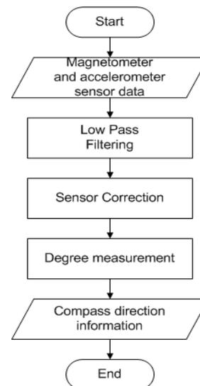
Fig. 2: Signal Processing model overview
