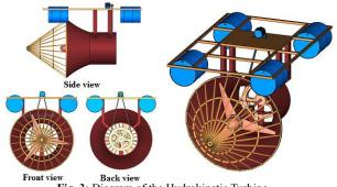
Fig. 3: Diagram of the Hydrokinetic Turbine.
