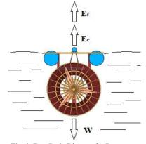
Fig. 4: Free-Body Diagram for Buoyancy.
