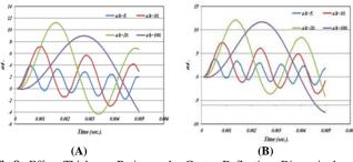
**Fig.8:** Effect Thickness Ratio on the Center Deflection, Dimensionless Normal Stresses and Transverse Shear Stresses as A Function of Time For Two Layered (0/90) Shells Subjected to Uniformly Distributed Triangular Pulse Load between (A)-Composite (M1) (B)-Hybrid (M2).
