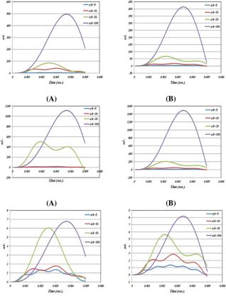
**Fig. 4:** Effect Thickness Ratio on the Center Deflection, Dimensionless Normal Stresses and Transverse Shear Stresses as A Function of Time For Two Layered (0/90) Shells Subjected to Sinusoidal Distributed Sine Pulse Load between (A)-Composite (M1) (B)-Hybrid (M2).
