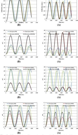
**Fig. 19:** Effect Number of Layered on Center Deflection and the Dimensionless Normal Stresses and Transverse Shear Stresses as A Function of Time for Two Layered (0/90) Shells Subjected to Uniformly Distributed Step Pulse Load between (A)-Composite (M1) (B)-Hybrid (M2).
