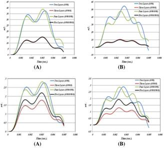
**Fig. 14:** Effect Number of Layered on the Center Deflection, Dimensionless Normal Stresses and Transverse Shear Stresses as A Function of Time for Two Layered (0/90) Shells Subjected to Sinusoidal Distributed Sine Pulse Load between (A)-Composite (B)-Hybrid.
