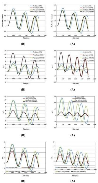
**Fig. 18:** Effect Number of Layered on the Center Deflection, Dimensionless Normal Stresses and Transverse Shear Stresses as A Function of Time for Two Layered (0/90) Shells Subjected to Uniformly Distributed Trian-
