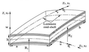
Fig. 1: Geometry of Laminated Spherical Shall Panel. [Ref. 10] the Strain-Displacement Relations Take the form [Ref. 5]
