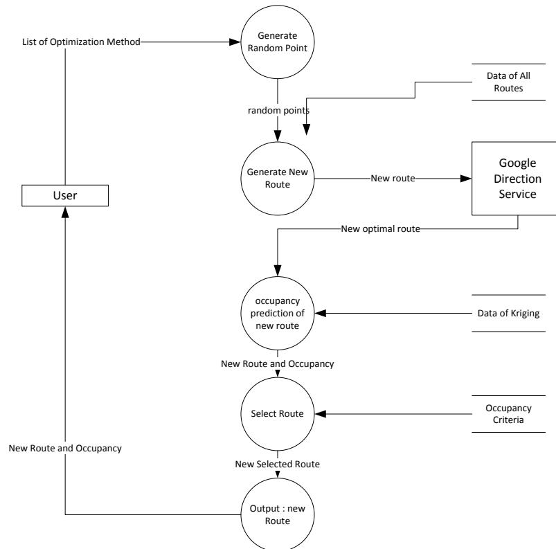
**Fig. 3:** DFD Optimal Route Recommendation
