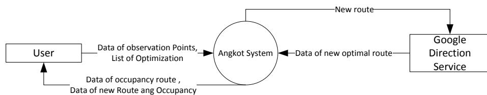
**Fig. 1:** Context Diagram of Public Transportation Routing System
