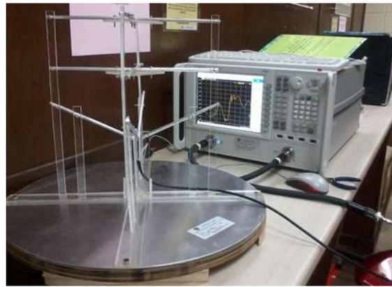
Fig. 6: Prototype of the 408 MHz antenna under measurement
