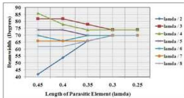
Fig. 4: Variation on beamwidth on the proposed 408 MHz antenna with two parasitic elements
