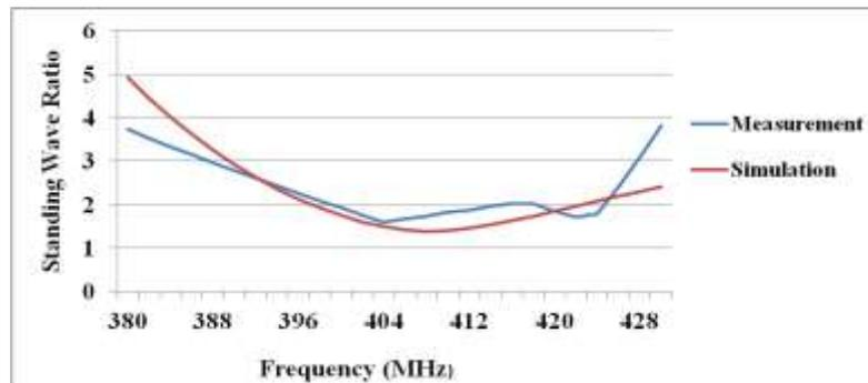
Fig. 7: Comparison on simulated and measured SWR of the 408 MHz antenna
