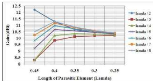
Fig. 5: Variation on gain on the proposed 408 MHz antenna with two parasitic elements
