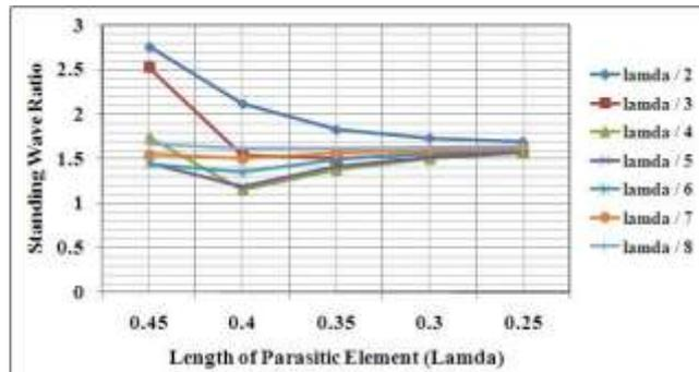
Fig. 3: Variation on SWR on the proposed 408 MHz antenna with two parasitic elements
