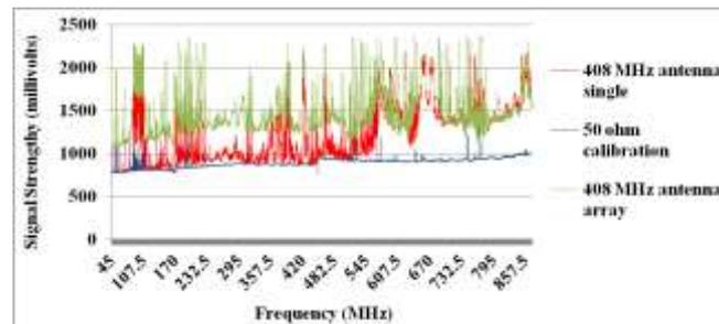
Fig. 8: Comparison on spectral views obtained by utilizing single antenna, array antenna and 50 ohm calibration
