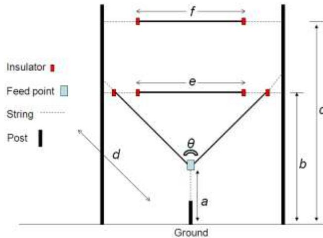
Fig. 1: Geometry of the proposed 408 MHz antenna
