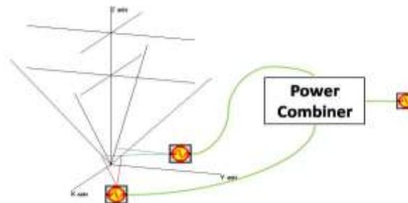
Fig. 2: Basic diagram of the dual-polarization V-shape dipole-based antenna
