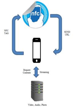
**Fig. 7:** Diagram of the NFC system-when an NFC equipped device is tagged to the NFC tag, prepared image, video and audio contents for the applying artifact are requested and then shown in the app
