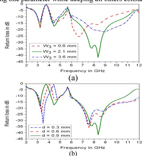
**Fig. 6.** Simulated return losses of proposed antenna for different (a) slot widths  $W_3$  (b) distance 'd'
