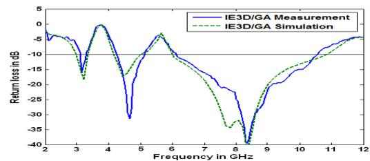
**Fig.5.** Return loss plots from IE3D/GA simulation and measurement
