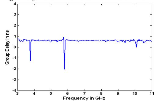
Fig. 9. Measured group delay response of the UWB antenna in the time domain
