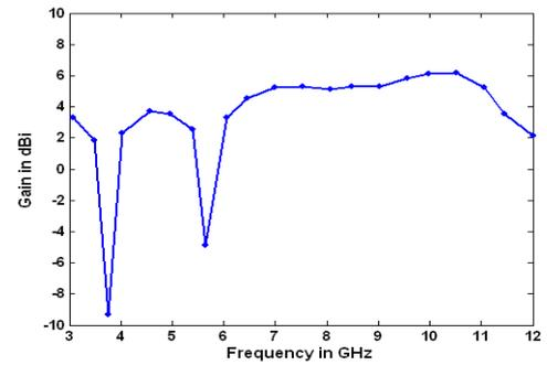
Fig. 8. Measured gain for the band notched antenna
