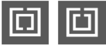
Fig. 1 (a) Rectangular CSRR (b) Co-directional CSRR
