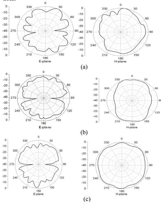
Fig. 7. Measured E and H-plane radiation pattern at (a) 3.2 GHz, (b) 4.7 GHz, (c) 8.3 GHz
