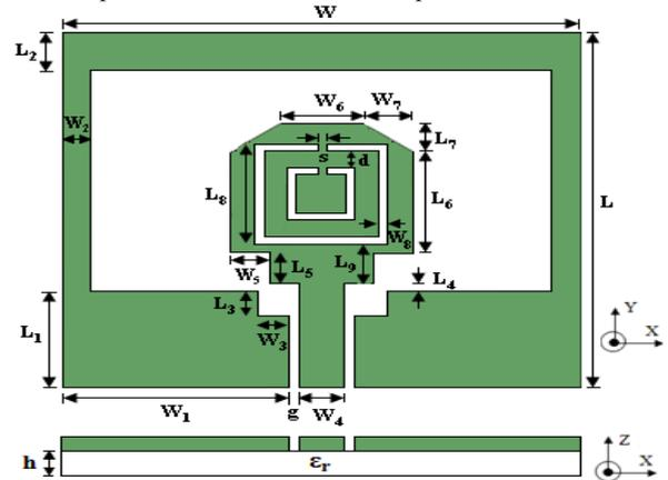
Fig. 2. Geometry of the proposed UWB slot antenna with co-directional CSRR
