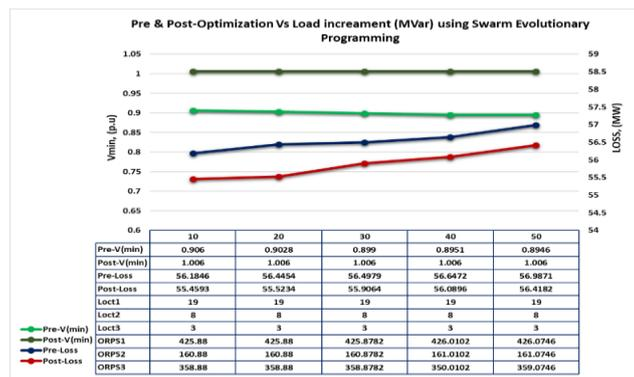
Fig. 4: Tabulated data of pre-optimization and post-optimization for voltage profile and total loss
