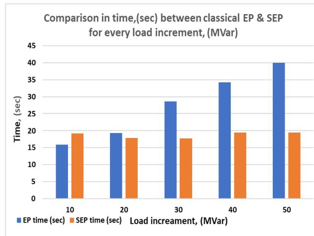
Fig. 5: Comparison of computational time results between EP technique and SEP technique.
