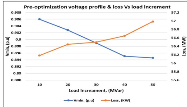
Fig. 3: Pre-optimization voltage profile and total loss versus load
