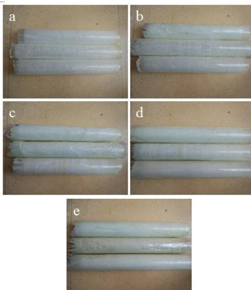
**Fig. 7:** The fabricated tubes with different layer of E-glass fibers: (a) one layer; (b) two layers; (c) three layers; (d) four layers and (e) five layers
