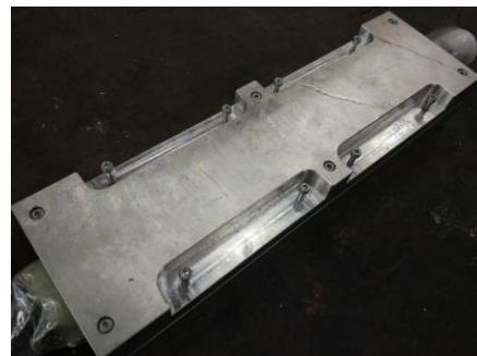
**Fig. 5:** The closed mold
