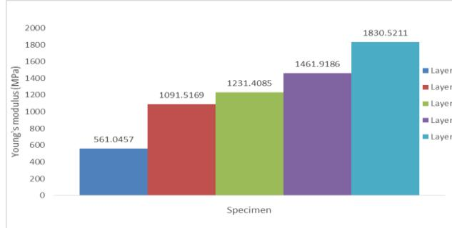
**Fig. 10:** Comparison of Young's modulus between the specimens with different layer of E-glass fiber in quasi-static crushing
