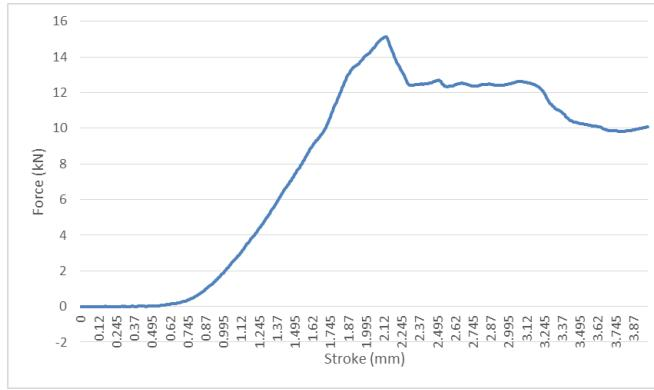
**Fig. 8:** Graph of Force versus Stroke for 4 layers of E-glass fiber (Test 2)
