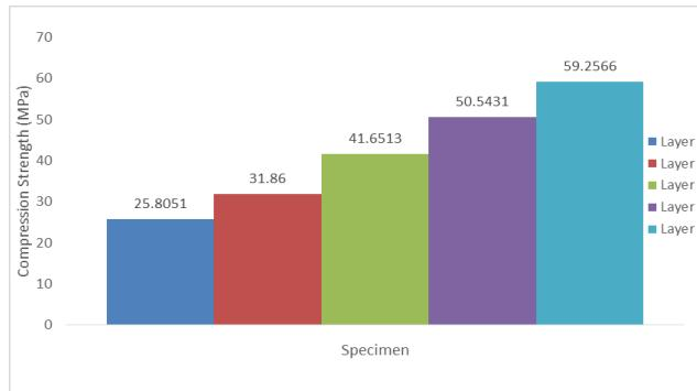
**Fig. 11:** Comparison of compression strength between the specimens with different layer of E-glass fiber in quasi-static crushing
