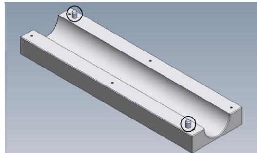
**Fig. 4:** Isometric view of the lower mold half with dowel pins
