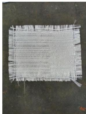
**Fig. 1:** E-glass fibers in mat form
