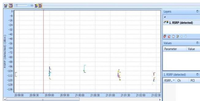
Figure 12: RSRP readings at 2F
