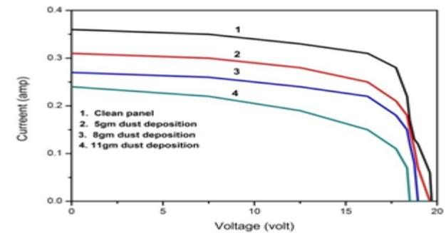
Fig. 2: I-V characteristic of PV module with lime stone dust deposition.
