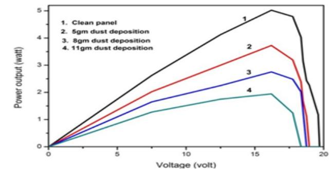
Fig. 3: P-V characteristic of PV module with red soil dust deposition.
