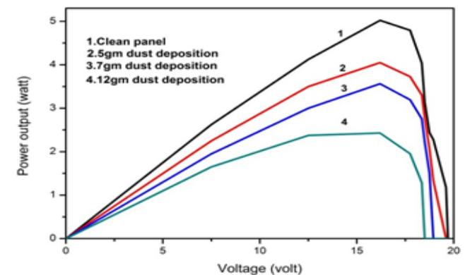
Fig. 4: P-V characteristic of PV module with lime stone dust deposition.
