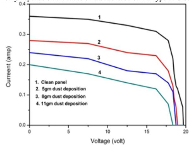
Fig. 1: I-V characteristic of PV module with red soil dust deposition.
