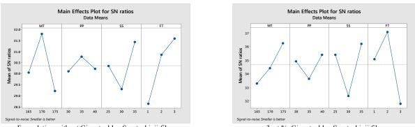
Formulation without Gigantochloa Scortechinii fibre 3 wt.% Gigantochloa Scortechinii fibre Fig.3: Signal to Noise Ratio (Shrinkage) for formulation without Gigantochloa Scortechinii fibre and 3 wt.% Gigantochloa Scortechinii fibre
