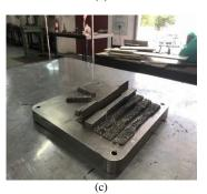
Fig. 5: Printed specimens from SLM process: (a) front view, (b) top view, and (c) isometric view
