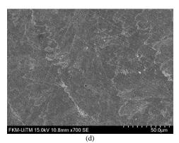
**Fig. 9**: SEM images from longitudinal view at the breaking point: (a) Sample P from rolled process, (b) Sample S from rolled process, (c) Sample T from SLM process and (c) Sample D from SLM process.
