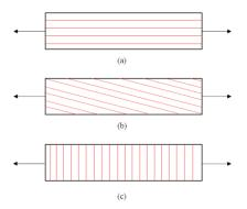
**Fig. 6**: Layer boundaries for SLM specimen according to build-up direction: (a) vertical, (b) horizontal with inclination angle and (c) horizontal without inclination angle.
