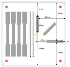
Fig 3: Dimension of the substrate plate.
