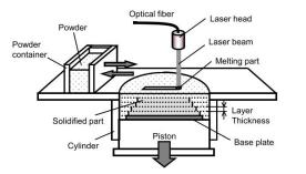
Fig. 1: Experimental equipment for selective laser melting process.
