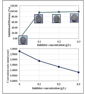
Fig. 3: Effect of inhibitor concentration to inhibition efficiency (IE) and corrosion rate (CR)
