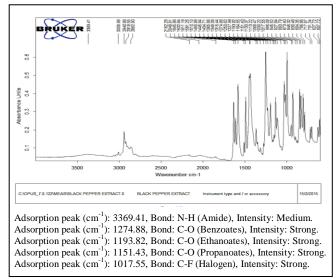
Fig. 2: FTIR Spectra for extraction of Piper Nigrum
