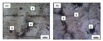
Fig. 4: Microstructure of Ductile Iron at 500 Times Magnification: (a) 0.1g/L Inhibitor Concentration (b) 0.3g/L Inhibitor Concentration. G: Graphite Nodule; F: Ferrite; P: Pearlite
