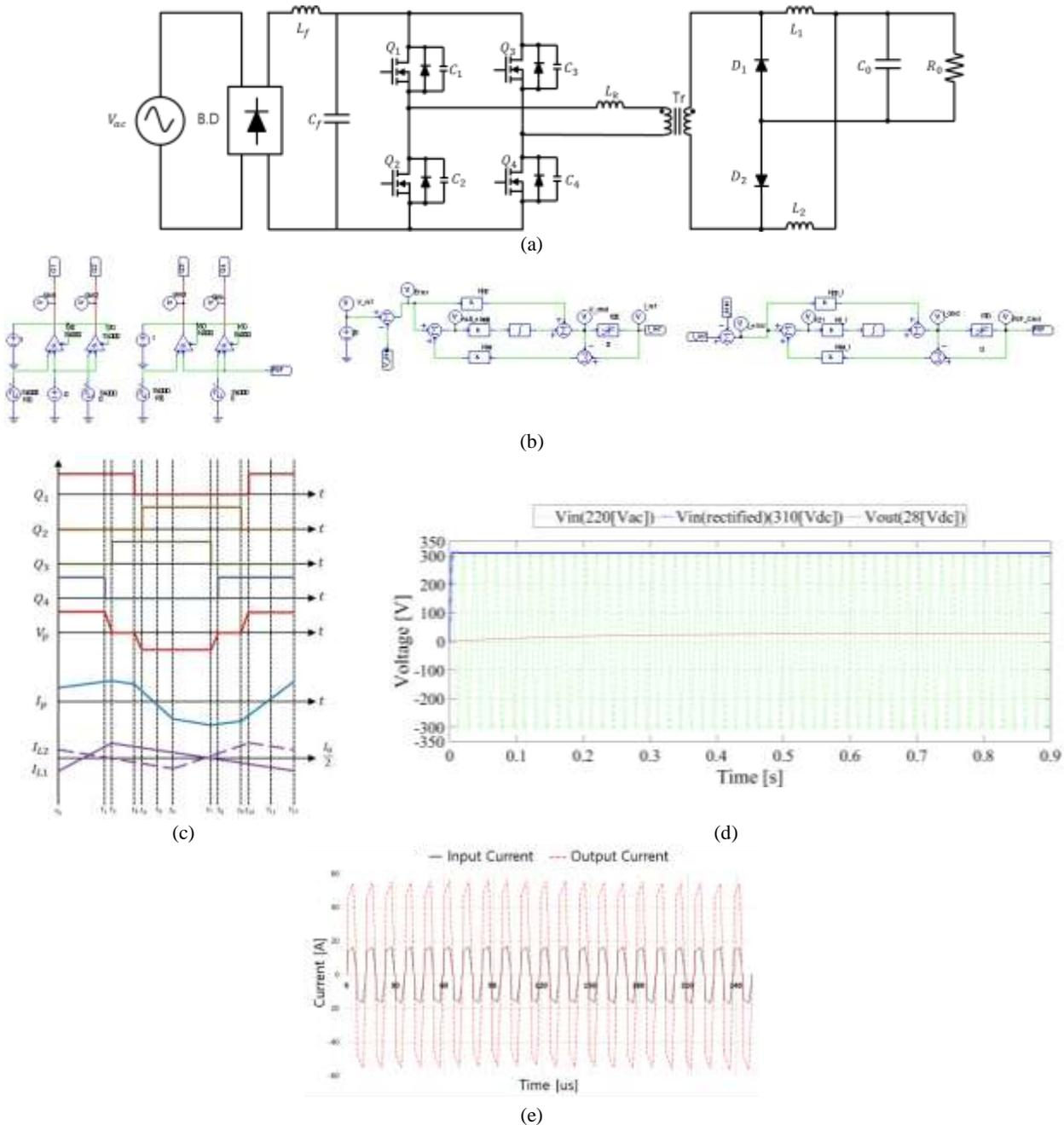
Figure 1: Circuit structure and simulation results of 3kW converter
