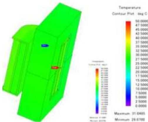
**Figure 5:** Results of the temperature distribution for a high frequency transformer core
