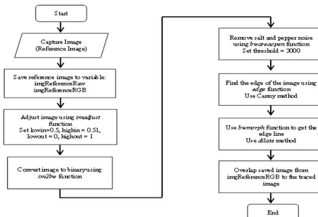
Fig. 6: Coral reef formation detection block diagram
