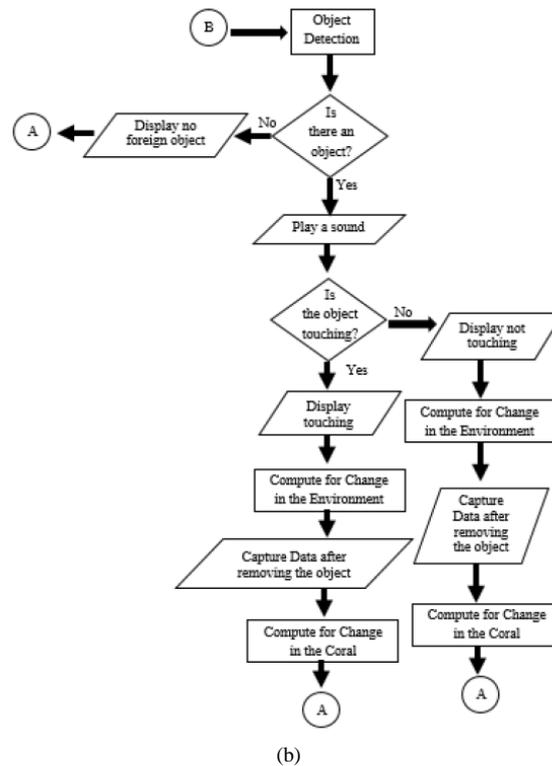
Fig. 2: (a) System Flow Chart Part 1, (b) System Flowchart Part 2
