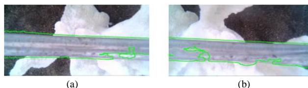
Fig. 10: Image differencing with a metal rod for (a) Camera A, (b) Camera B
