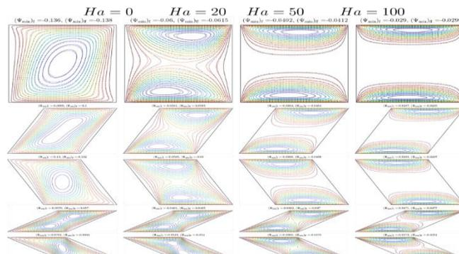
**Fig. 2:** Variations of the isotherms evolution by Hartmann number  $Ha$  left to the right and inclination angle of the sloping wall  $\varphi$  top to the bottom for  $Gr = 10^4$ ,  $\phi = 0$  (solid lines) and  $\phi = 0.03$  (dashed lines).
