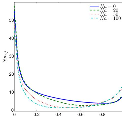
**Fig. 4:** Variations of local Nusselt numbers interface with  $Y$  for different  $Ha$  at  $\phi = 30$   $Gr = 10^4$  and  $\phi = 0.03$ .
