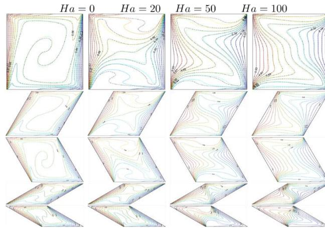
**Fig. 3:** Variations of the isotherms evolution by Hartmann number  $Ha$  left to the right and inclination angle of the sloping wall  $\phi$  top to the bottom for  $Gr = 10^4$ ,  $\phi = 0$  (solid lines) and  $\phi = 0.03$  (dashed lines).
