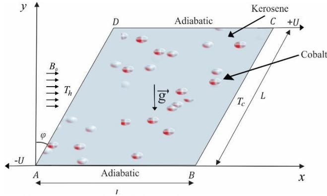
**Fig. 1:** Physical model of convection in an oblique cavity together with the coordinate system.
