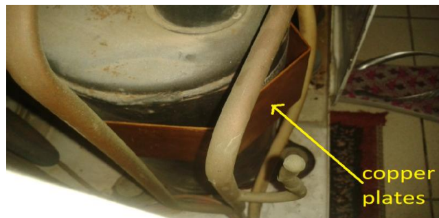
Fig. 4: Copper Plate for TEG Array mounted on the AC Compressor
