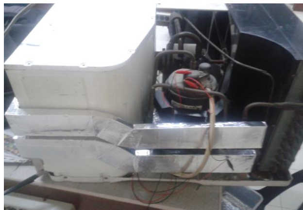
Fig. 5: Cooling System attached to Air Conditioning Unit's Air Duct and Heat Sinks
