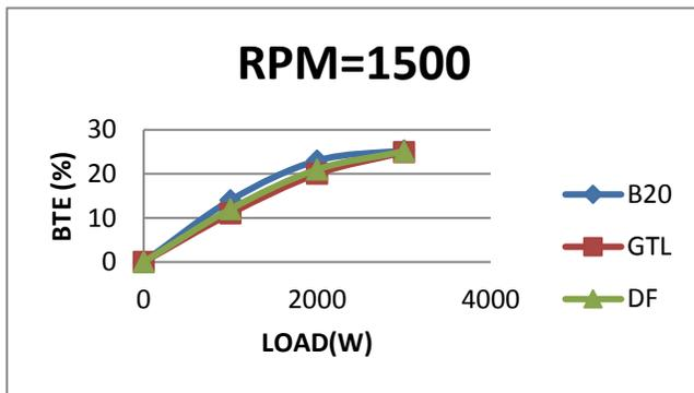
Fig: 3: Variation of BTE with load
