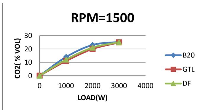
Fig. 8: Variation of CO<sub>2</sub> with Load
