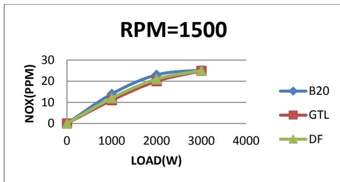
Fig. 7: Variation of NOx with Load
