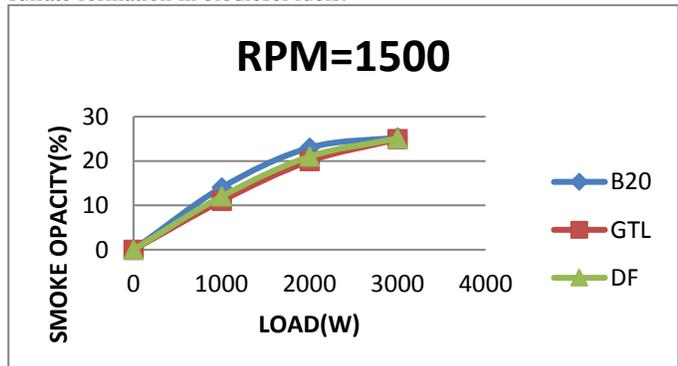
Fig. 9: Variation of Smoke with Load
