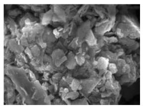
Fig 4.9: SEM Image of Copper Slag
