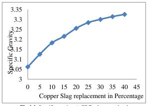
Fig 4.4: Specific gravity v/s CS Replacement level
