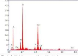
Fig 4.13: EDS Spectrum of 25% CS with Cement
