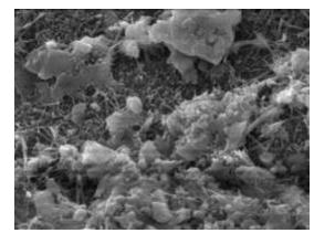
Fig 4.12: SEM Image of 25% CS with Cement
