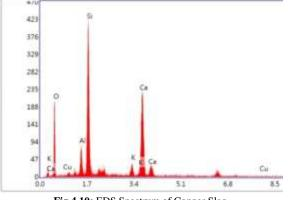
Fig 4.10: EDS Spectrum of Copper Slag
