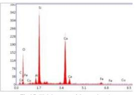
Fig 4.7: EDS Spectrum of Cement Sample
