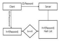
Figure 4: Password based Authentication Model Using One-Way Function
