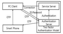
Figure 5: Smart Phone Based Authentication
