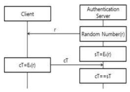
Figure 2: Challenges-Response Based Authentication Model
