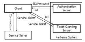
Figure 3: Kerberos System Based Application Model
