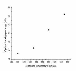
Fig. 7: Optical band gap differentiation between all ZnO nanostructures films
