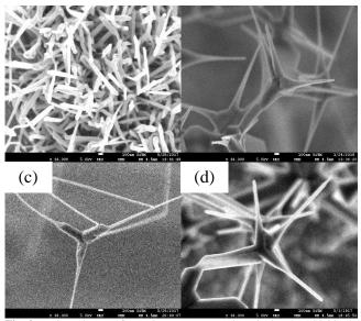
Fig. 2: FESEM images for ZnO nanostructure deposited at (a) 500 °C, (b) 550 °C, (c) 600 °C and (d) 650 °C
