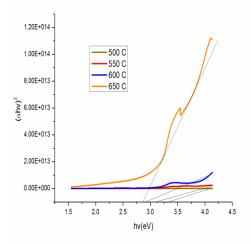
Fig. 6: Optical band gap for ZnO nanostructures film calculated using Tauc method
