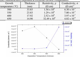
Fig. 3: Resistivity and conductivity values obtained from I-V measurement
