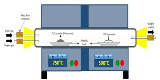
Fig. 1: TCVD with two double furnace system used to deposit ZnO nanostructures  $% \left( {{{\mathbf{T}}_{{\mathbf{N}}}} \right)$
