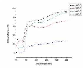
Fig. 4: Transmittance spectra for all ZnO nanostructures deposited
