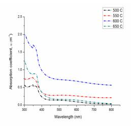
Fig. 5: Absorption coefficient ZnO nanostructures deposited at various temperatures
