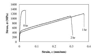
Fig. 4: Stress-strain curves of rolling sample with gas carburizing for 1 and 2 hours.
