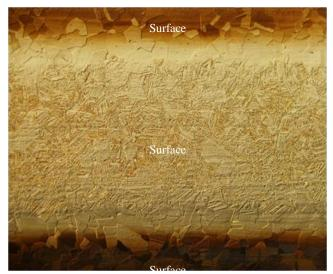
Fig. 11: Carburized layer of Fe-24Mn steel (austenite at the surface).
