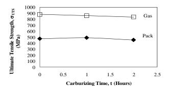
Fig. 7: Ultimate tensile strength of Fe-24Mn steel samples before and after carburizing.
