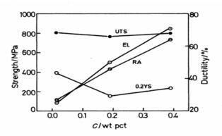
Fig. 9: Tensile properties of Fe-24Mn alloys with different C content [22].
