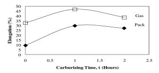
Fig. 8: Elongation of Fe-24Mn steel samples before and after carburizing.
