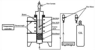
Fig. 1: Schematic diagram of the gas carburizing process [14]
