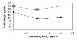
Fig. 6: Yield strength of Fe-24Mn steel samples before and after carburizing.
