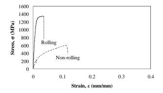
Fig. 3: Stress-strain curves of rolling and non-rolling sample before carburizing
