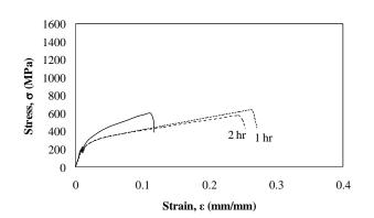
**Fig. 5:** Stress-strain curves of non-rolling sample with pack carburizing for 1 and 2 hours.
