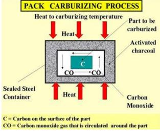
Fig. 2: Schematic diagram of the pack carburizing process [18]
