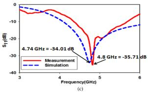
**Fig. 4**: Simulated and measured reflection coefficient, S11 of cylindrical monopole plasma antenna. (a) Argon gas. (b) Neon gas (c) Hg-Ar gas
