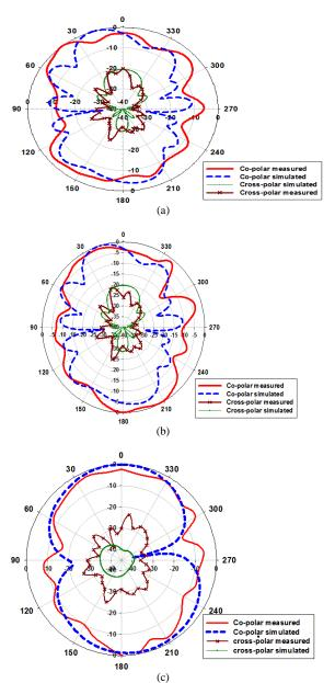
Fig. 5: Simulated and measured radiation patterns. (a) Argon gas (b) Neon gas (c) Hg-Ar gas
