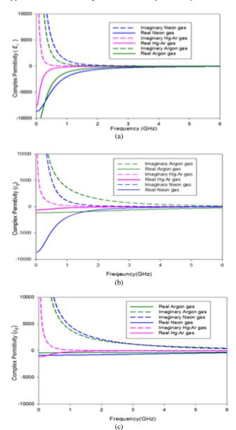
Fig. 2: Relative Permittivity for argon gas, neon gas and Hg-Ar gas for (a) 0.5 Torr (b) 5 Torr and (c) 15 Torr.
