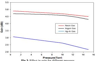
Fig.3: Effect in gain for different pressure
