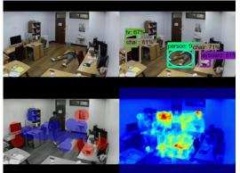
Fig. 16: Unusual stationary behavior in an infrequent location and detection using our vision classifier.
