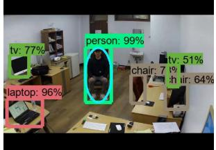
Fig. 12: Human and object detection in a normal life using our vision classifier.
