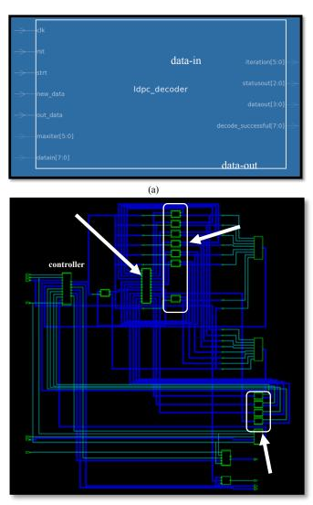
(b) **Fig. 6.** Main LDPC decoder: (a) Module (b) Internal
