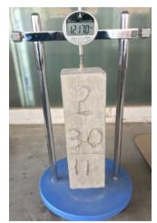
Fig. 8: Digital Length Comparator Apparatus with Specimen for testing
