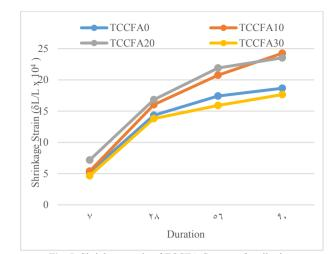
Fig. 5: Shrinkage strain of TCCFA Concrete for all mixes
