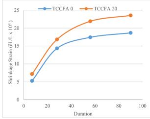
Fig. 3: Comparison of Shrinkage strain of Concrete for TCCFA 0 and TCCFA 20  $\,$
