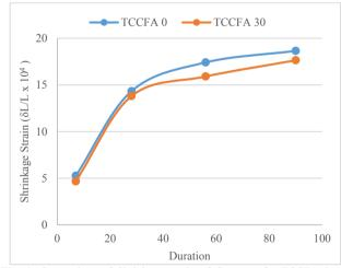
Fig. 4: Comparison of Shrinkage strain of Concrete for TCCFA 0 and TCCFA 30  $\,$
