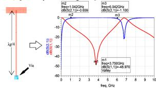
Fig.3 λg/4 short circuited stub layout and ADS Simulation Response.
