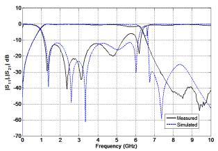
Fig.5 (b) Case-II: Simulated and measured BPF performance
