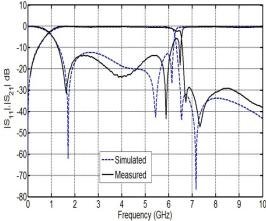
Fig. 4 (b) Case-I: Simulated and measured BPF performance
