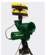
Fig. 12: Pneumatic Bowling Machine.
