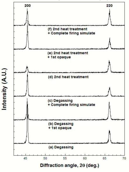
Fig. 7: Change in the XRD pattern during simulated porcelain firing
