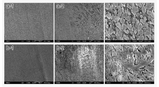
Fig. 5: Microstructural changes during simulated porcelain firing: (a) degassed, non-heat treated specimen (b) degassed, heat treated specimen At magnifications of x2000 (1), x6000(2), x30000(3)
