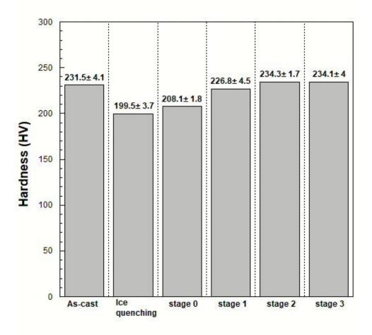
Fig. 3: Hardness change of specimens by cooling stage after simulated porcelain firi
