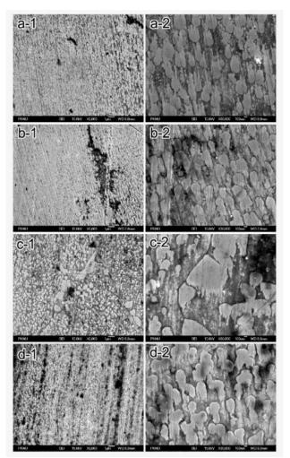
Fig. 6: Microstructural changes during simulated porcelain firing: (a) 1st opaque stage, non-heat treated (b) 1st opaque stage, heat treated (c) add-on stage, non-heat treated (d) add-on stage, heat treated At magnifications of x6000 (1), x30000(2)
