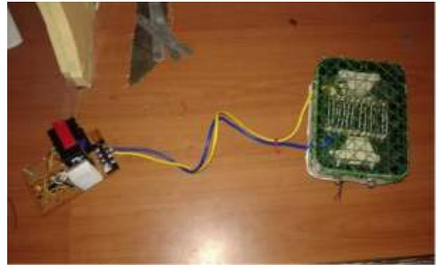
Fig. 2: Buck Converter Along with the Dynamic Load.
