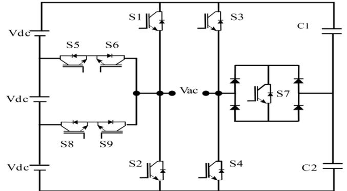
Fig. 3: The Proposed MANPC Converter Topology.
