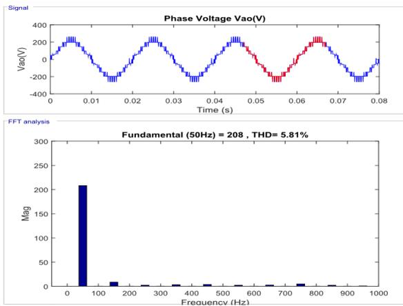
Fig. 7: Output Phase Voltage and Harmonic Spectra for  $M_A = 0.6$  with THD Value 6.81%.
