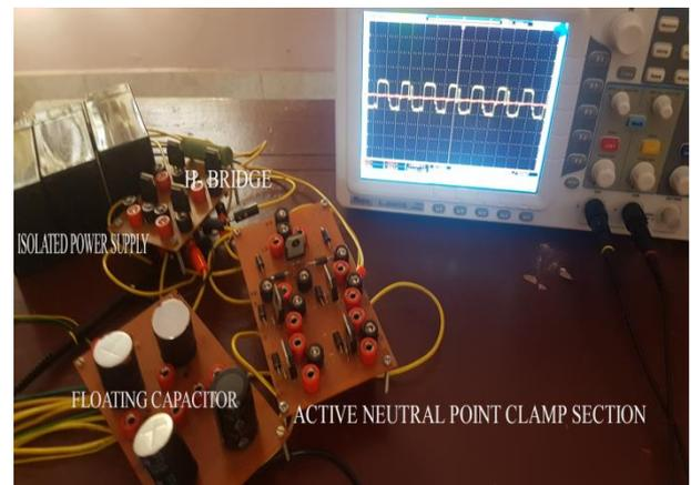
Fig. 16: Hardware Prototype of the Proposed MANPC Converter.
