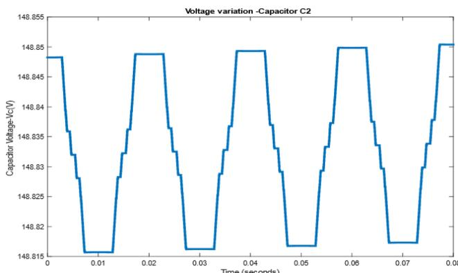
Fig. 14: Charging and Discharging Cycles of Capacitor C2.
