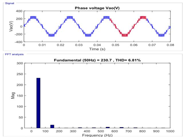
Fig. 15: Output Phase Voltage and Harmonic Spectra for  $M_A = 1$  with THD Value 5.60%.
