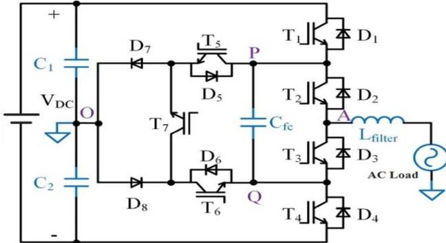
Fig. 2: An NPC Five Level Seven Switch Topology.
