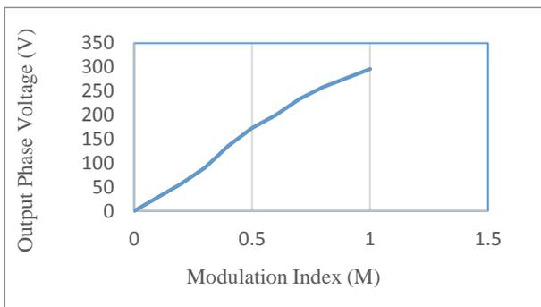
Fig. 13: Fundamental Output Voltage vs. Modulation Index.
