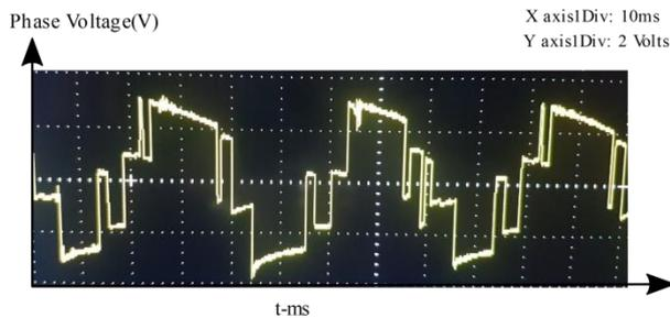
Fig. 17: Output Phase Voltage of 36 V System with Modulation Index  $M_A = 0.2$ .
