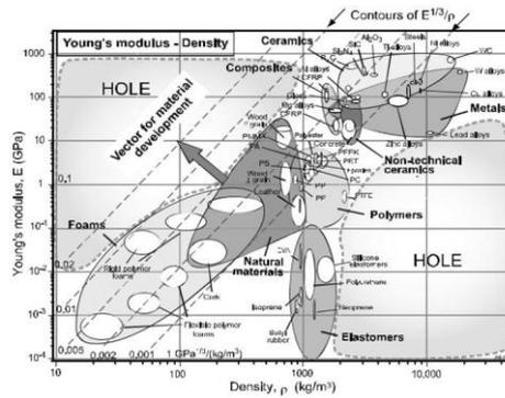
Fig. 1: Lattice structure has the potential to fill in holes in Young's modulus and density graph [8]
