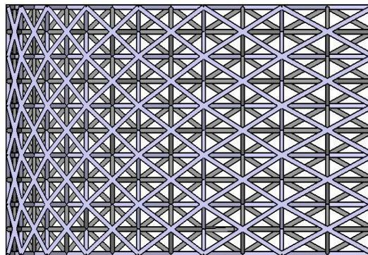
Fig. 14: Octet-truss lattice structure in a single gradient direction
