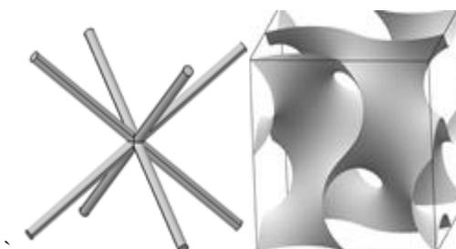
**Fig. 6:** (a) BCC and (b) gyroid [20] elementary structure
