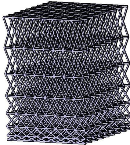
Fig. 13: 90° FCCZ structure varied in one direction unit cell length
