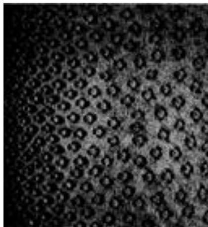
Fig. 3: Microstructure of cross section for bamboo [13]
