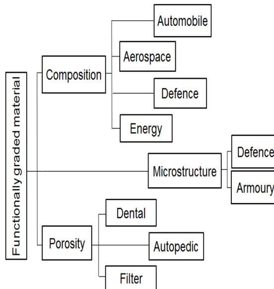
Fig. 2: Functionally graded material application classification [13]
