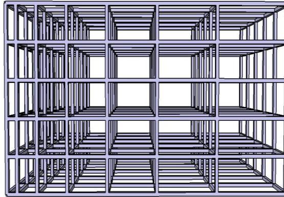
Fig. 10: Gradient cubic lattice structure variation in y-direction
