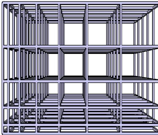
Fig. 11: Gradient cubic lattice structure variation in y and z-direction
