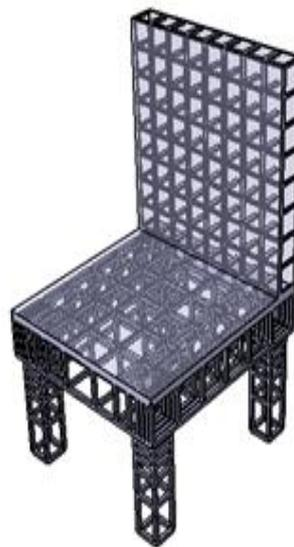
Fig. 12: Smaller unit cell is located at the higher force area of the chair
