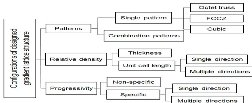
Fig. 5: Proposed design configurations of gradient lattice structure
