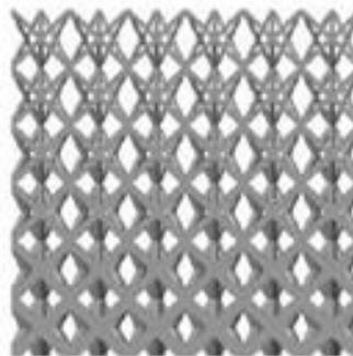
Fig. 9: F2BCC lattice structure with varied strut dimensions [6]
