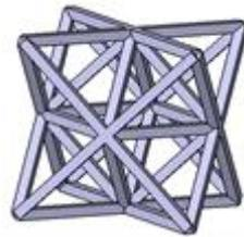
Fig. 8: Octet-truss pattern
