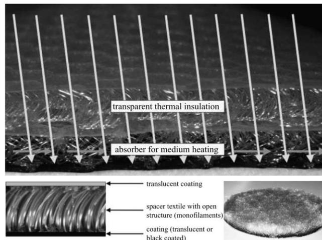
Fig. 5: Thermal insulation textile composites [41].
