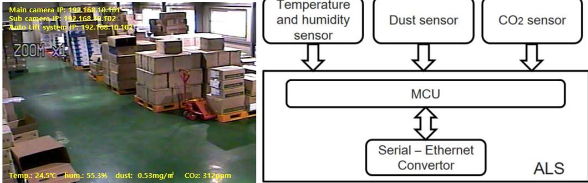
Figure 6. Display of data from sensors on screens and sensor hardware composition using ALS
