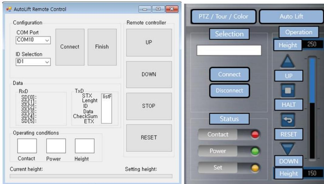
**Figure 4.** ALS control program a) Independent type b) NVR-integrated type
