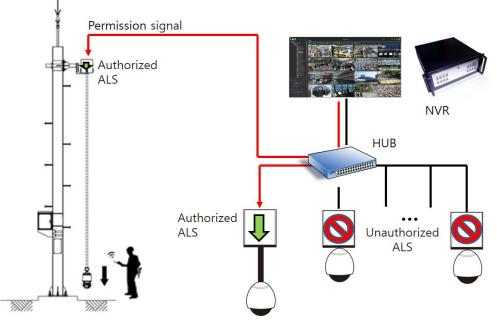
Figure 3.ALS and CCTV cameras controlled by NVR
