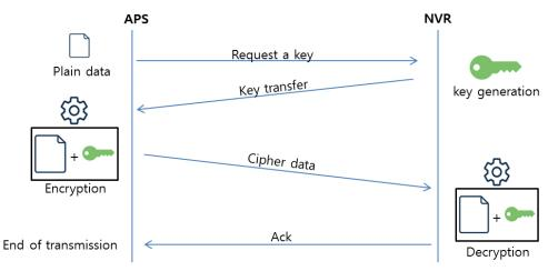
Figure 7. Communication procedure between ALS and NVR using encrypted key
