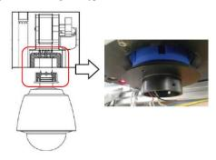
Figure 5. Lower socket detached inside the ALS
