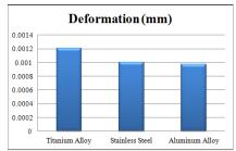
Figure 11: Deformation of different blade materials @ 40000RPM
