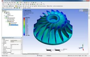
Figure 13: Strain distribution of micro turbine compressor blade
