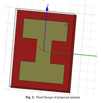
If the impedance is matched properly, the results obtained will have good return loss of around -10dB to -35dB and a VSWR in between 1-2dB. In HFSS the far field radiations are also shown by plotting the Radiation pattern in 2D or 3D. HFSS uses Finite Element Method, with adaptive meshing, and good graphics to give best results for all of the 3D EM problems [7].
