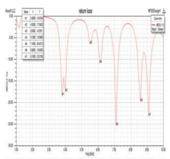
Fig. 3: Return loss VS Frequency plot in HFSS
