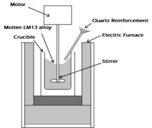
**Fig 2:** Stir casting setup.
