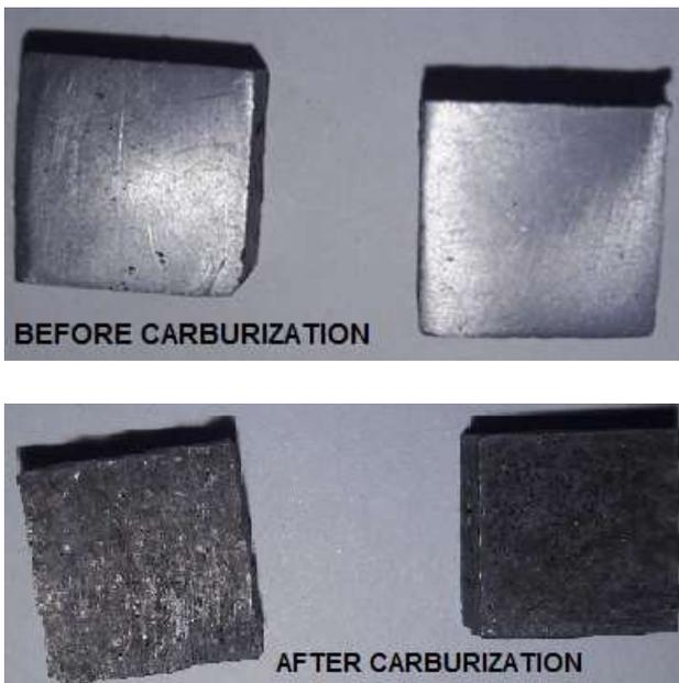
Fig5: Specimens before and after carburization.
