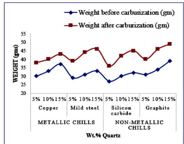
Fig7: Specimen weight before and after carburization carried out for 90 hours.
