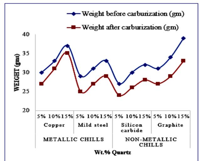
Fig8: Specimen weight before and after carburization carried out for 120 hours.
