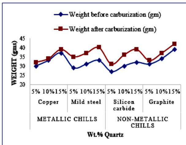
Fig6: Specimen weight before and after carburization carried out for 60 hours.
