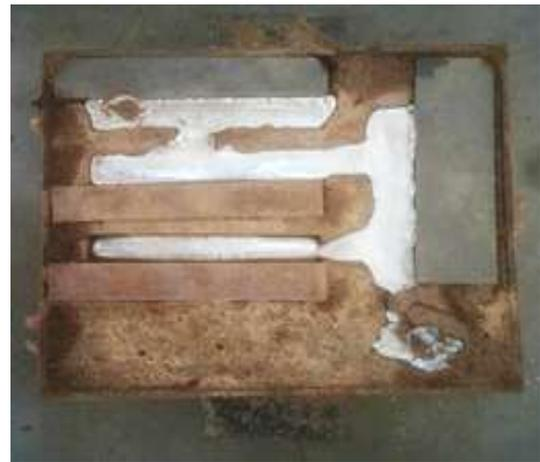
**Fig 3:** Placement of end chills in the mould.
