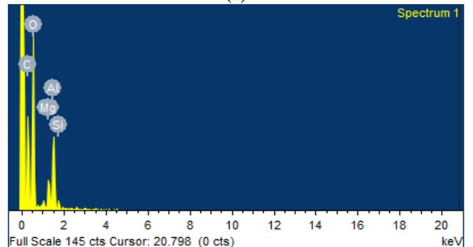
Fig11: EDX for specimen carburized for 90 hours; (a) SEM of the oxide layer; (b) EDX
