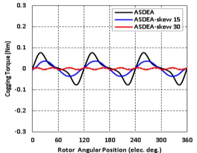
Fig. 6: Cogging torque of PMSM before and after stator skewing
