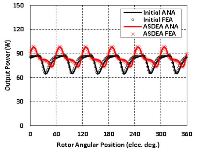
Fig. 5: Output Power of PMSM before and after optimized
