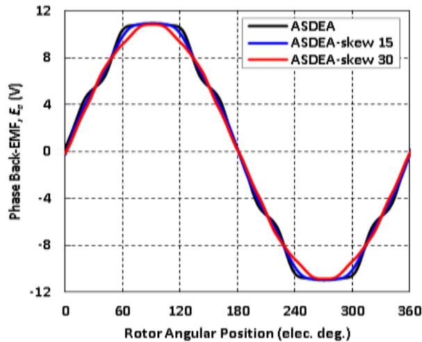
Fig. 7: Phase back-EMF of PMSM before and after stator skewing
