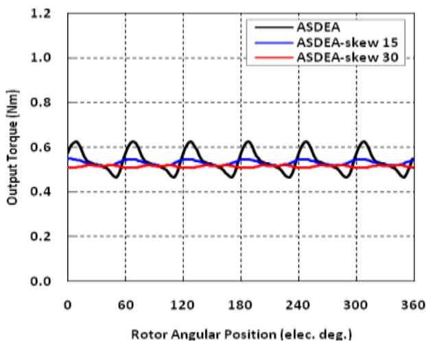
Fig. 9: Output torque of PMSM before and after stator skewing
