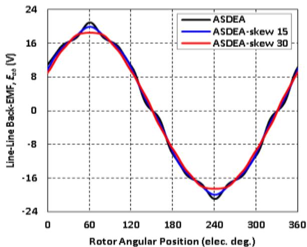
Fig. 8: Line-line back-EMF of PMSM before and after stator skewing
