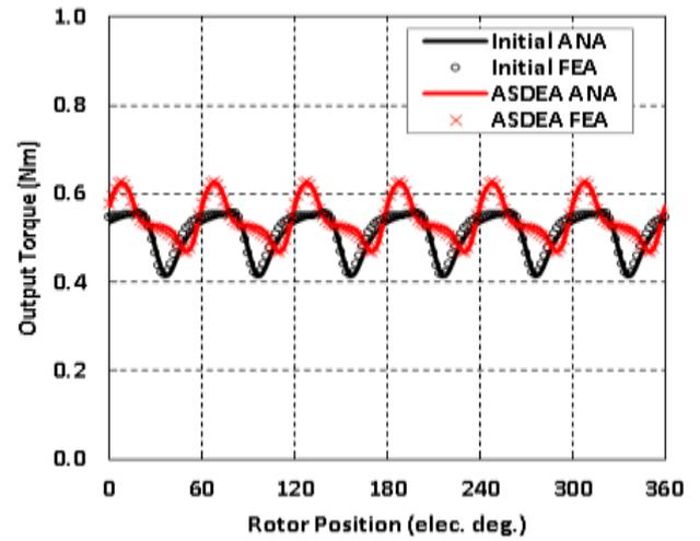
Fig. 4: Output torque of PMSM before and after optimized.
