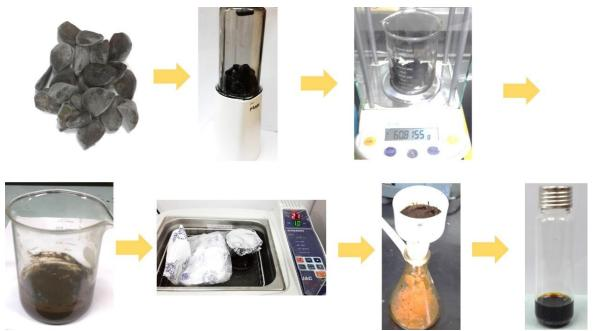
Fig. 1: Sample preparation process of black garlic (mixing water, sonication, and filtration). The final filtrate was moved to headspace vial for the GC-FID static headspace injection
