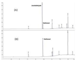
Fig 3: The GC-FID chromatogram separated on CP-poraPLOT U column for (A) raw garlic and (B) black garlic sample
