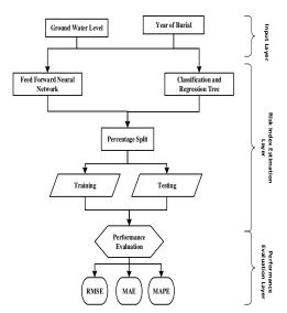
Figure.1: Proposed Risk Index Estimation Methodology in Underground Metro Structure
