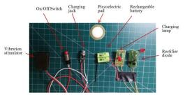
Figure 7: Electronic devices for Manufacturing Vibration stimulators
