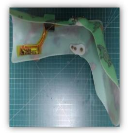
f) Orthosis with vibration stimulator **Figure 8:** Manufacturing process of Ankle-foot orthosis with Vibration stimulator
