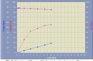
Fig.3: Variation of Torque, Mechanical and volumetric efficiency
