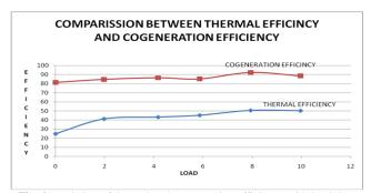
Fig. 4: Variation of thermal and cogeneration efficiency with load (kg)
