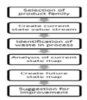
Fig. 1: Methodology of VSM implementation in ABC Pvt. Ltd. for AL-PHA1 process line
