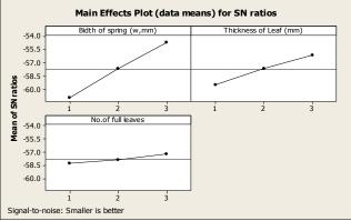
**Fig 8:** Signal/Noise ratio analysis of deflection of leaf spring at 60kmph in h2 road condition
