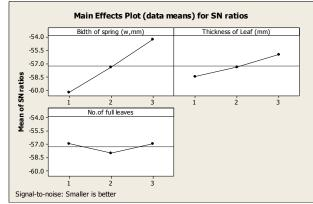
Fig 6: S/N ratio analysis of deflection of leaf spring at 60kmph in h1 road condition
