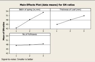
Fig 7: Signal/Noise ratio analysis of total stress of leaf spring at 60kmph in h2 road condition
