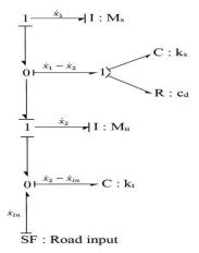
Fig. 3: BG model (Bond Graph) of 2-DOF quarter car suspension system
