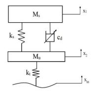
Fig. 2: 2-DOF quarter car model with controllable damper
