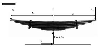
Fig 1: Forces acting on Leaf spring
