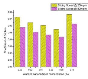
Figure 2: Effect of nanoparticles concentration on COF.
