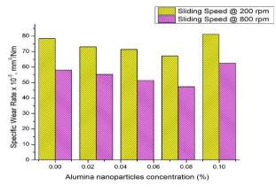
Figure 4: Nanoparticles concentration on specific wear rate.
