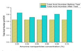
Figure 5: Total acid number with different alumina concentration percentage
