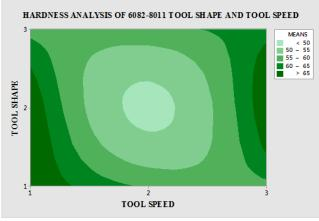
Fig. 3: Contour curves of tool shape and tool speed
