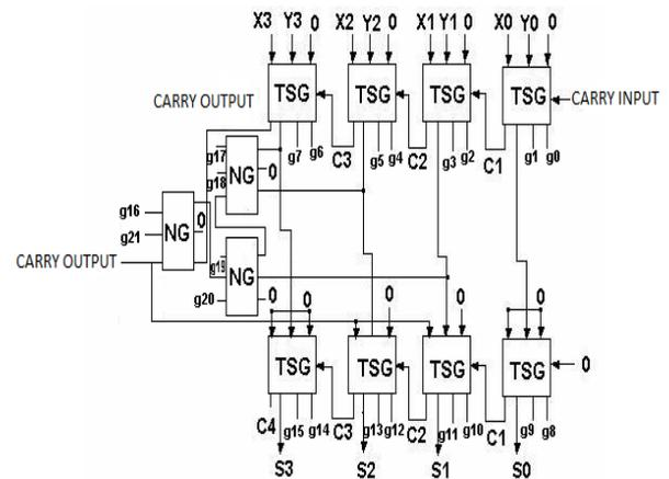
Fig.5: Complimentary implementation of conventional BCD adder
