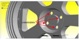
Fig. 4: Constraint applied to bolt holes
