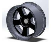
Fig. 2: Isometric view of a 3D model design of an automobile alloy wheel
