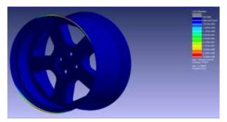
Fig. 7: Number of cycles to failure for aluminium alloy wheel
